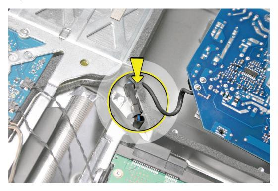
4. Connect the DC power cable and the ground cable to the underside of the power supply.
